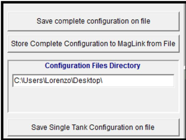
Once the configuration of the console has been completed, it is possible to do a backup of the console parameters clicking "Save complete configuration on file" button.
