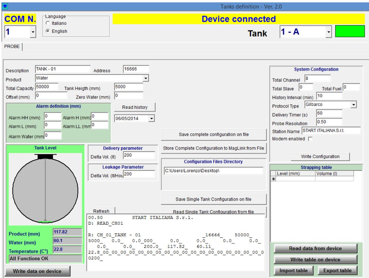
For each tank user must set appropriate parameters.
