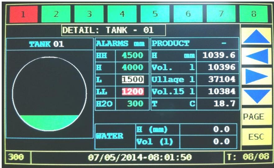
To ack an alarm press ESC button, beep will stop.
