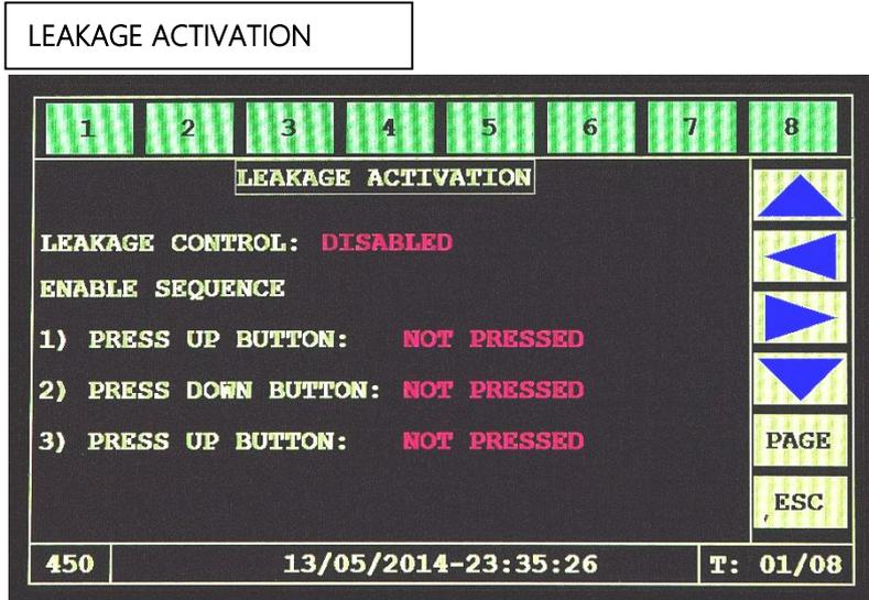
Leak detection procedure is based on an algorithm which monitors the tank. It is mandatory that no external movements occur during the activation period.
